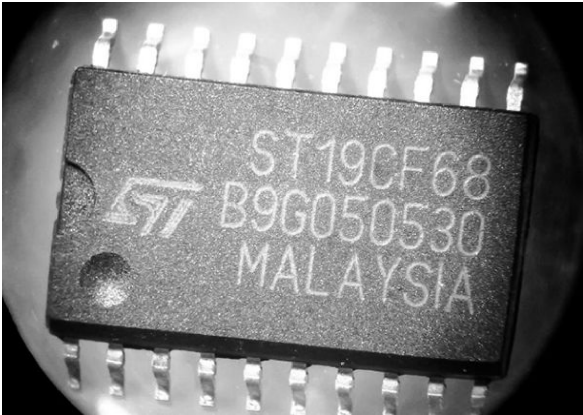
A close-up of the outside of the fake ST19CF68
