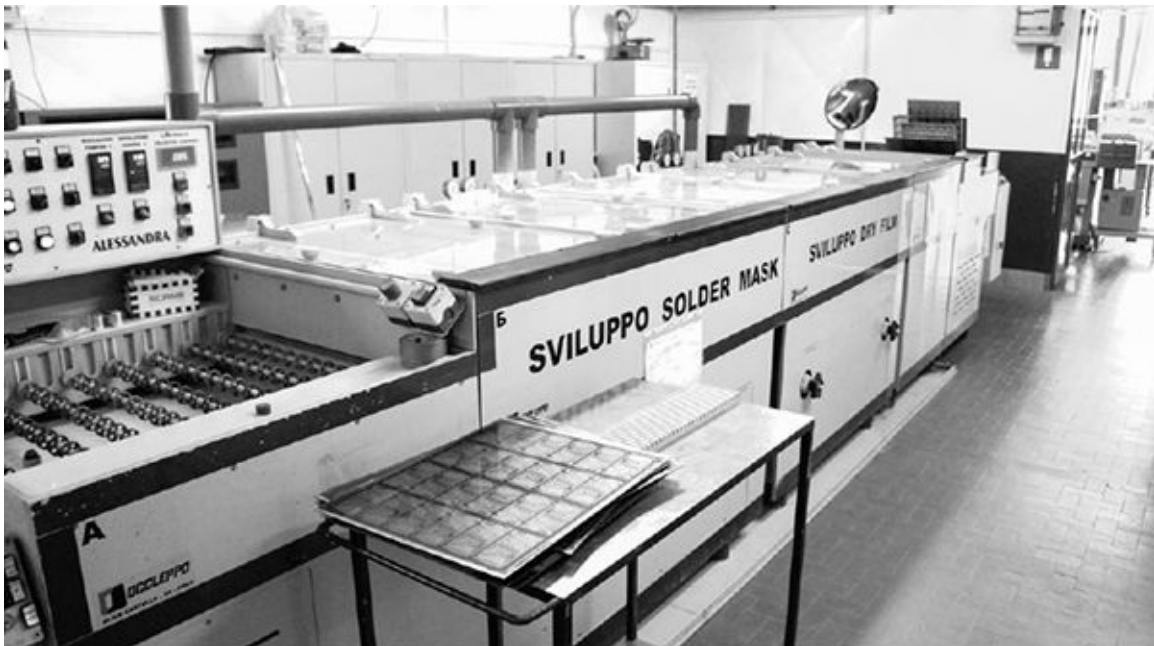
The machine that develops the photoresist
