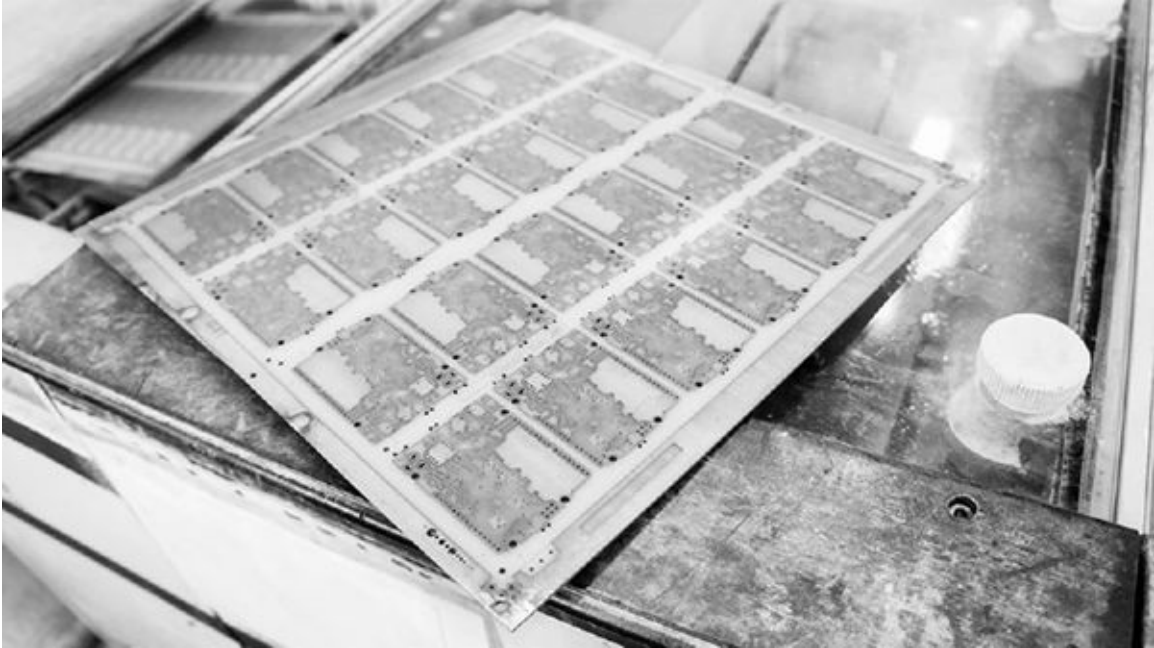
A panel etched of unwanted copper
