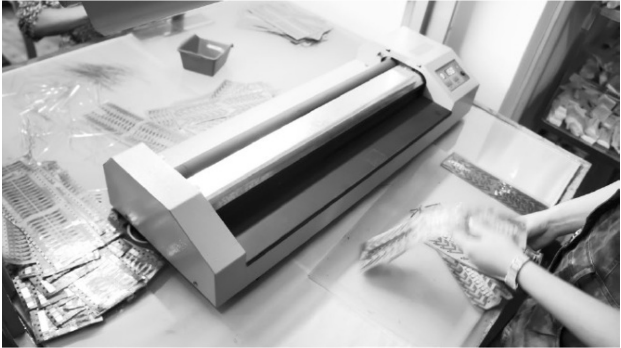
Steel plates being laminated to the back of flex-circuit material
