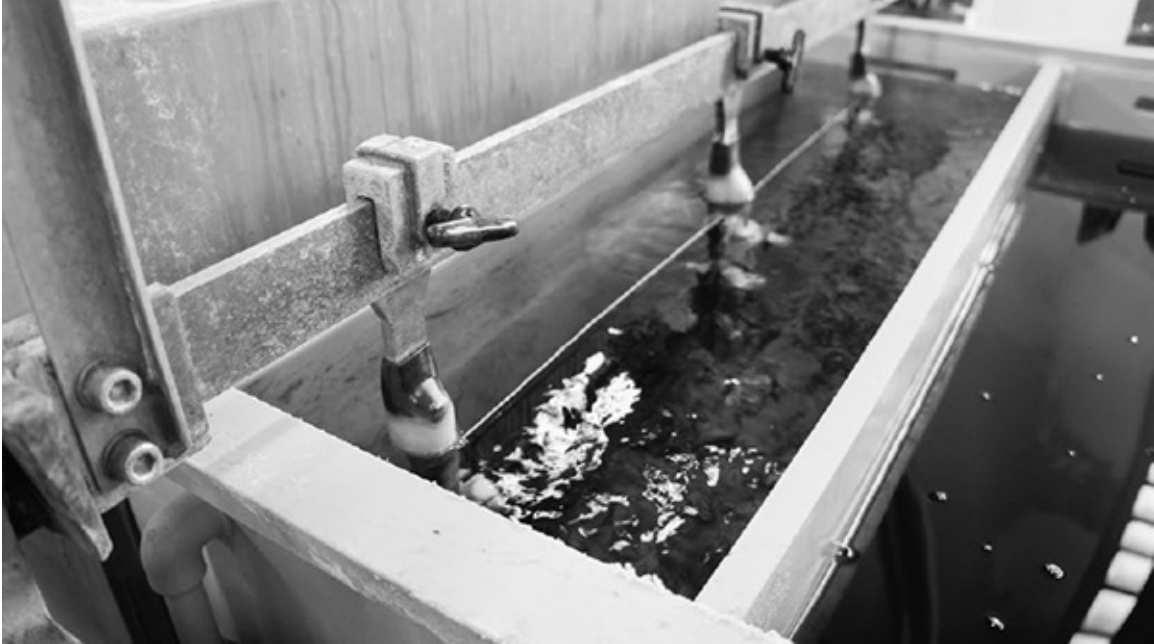
A machine that moves panels around in etchant
