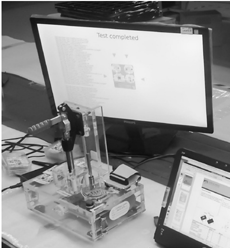
The testing machine for the Chibitronics microcontroller sticker
