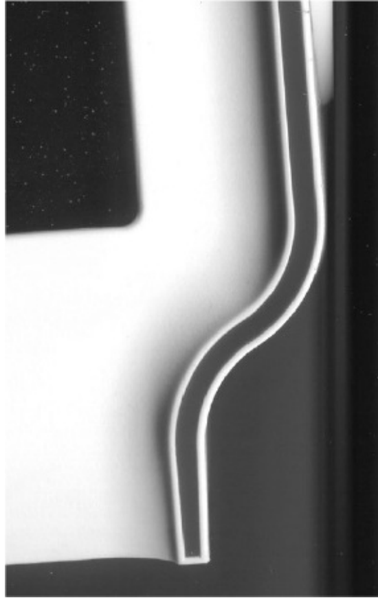
A perfect chumby One ridge, from the double-injection mold process
