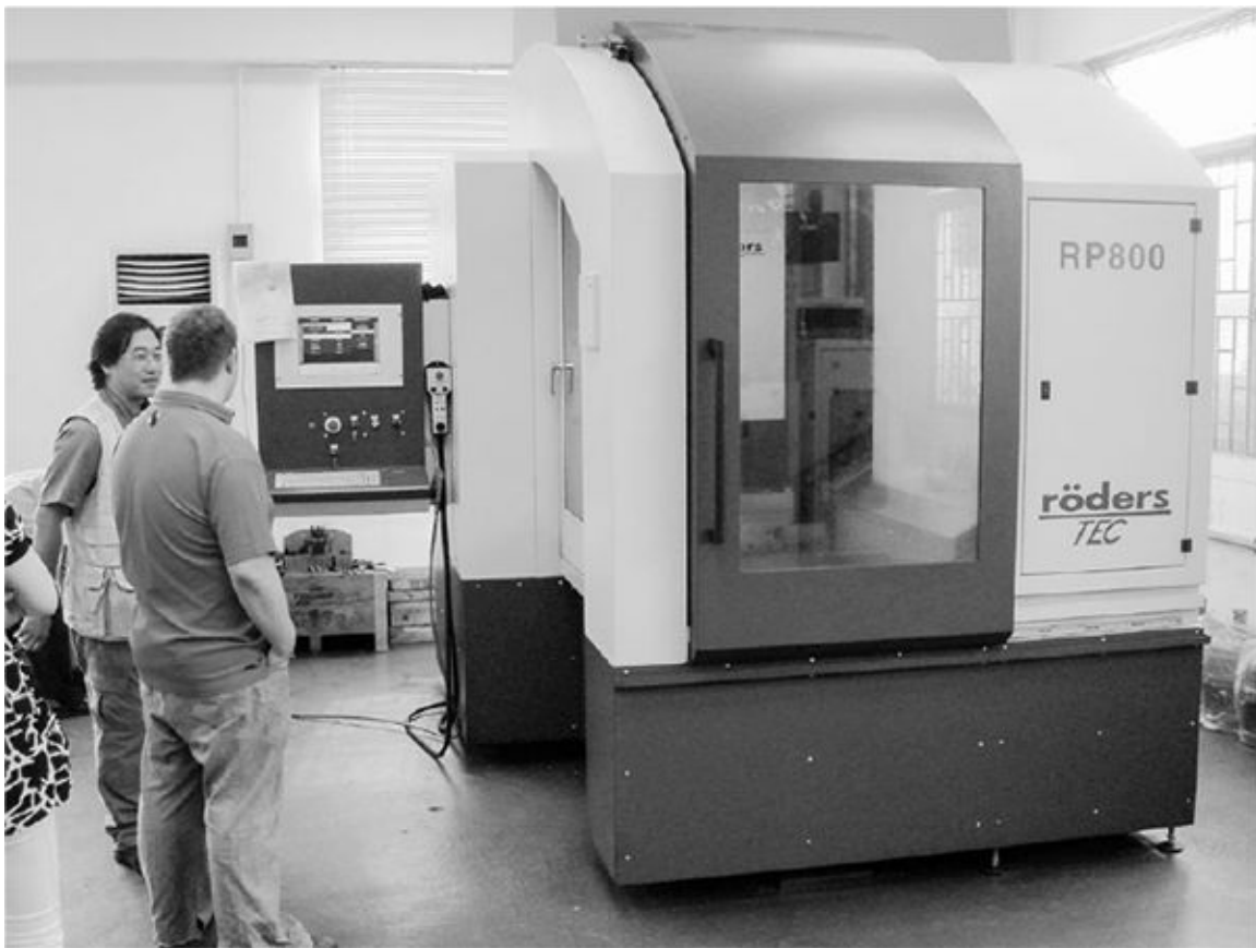
The mold-cutting machine used in manufacturing chumbys. Compare it to the people standing next to it for scale.
